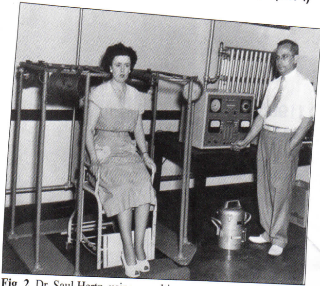
Fig. 2. Dr. Saul Hertz, using a multicounter to analyze the distribution of radioactive iodine in a patient in early 1941.
